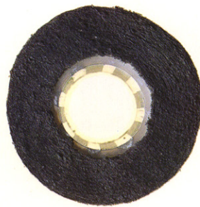
A section through a Profile II filter element showing the effective use of the full depth of the element.
