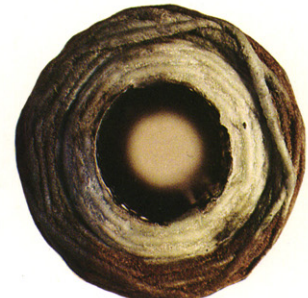
A section through a competitor's filter showing only partial usage before the element needed to be changed.
